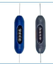
The frequency of the flashing LEDs indicates the voltage level on the fence. The longer the period between flashes, the lower the voltage on the fence. The intensity of the light remains the same so it can be seen from far irrespective of the fence voltage. It is installed between the earth and live wire to indicate the status and condition of the fence for peace of mind.
